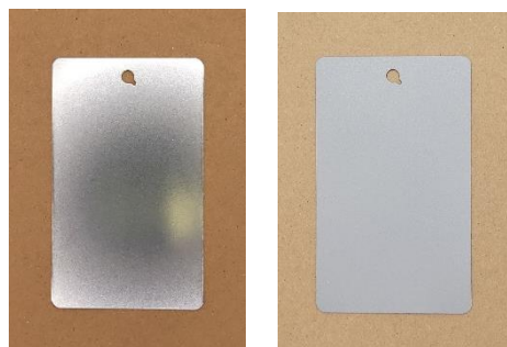
The plate on the left is blasted not blasted and looks shiny and smooth. The plate on the right is blasted and looks dull and rough. That is what you are looking for.
