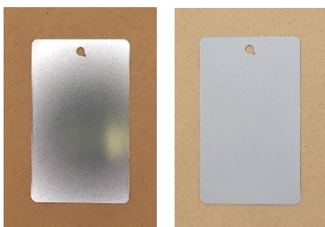
The plate on the left is blasted not blasted and looks shiny and smooth. The plate on the right is blasted and looks dull and rough. That is what you are looking for.
